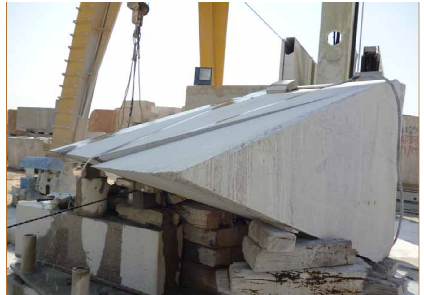
Works on statue shape by diamond wire (Workshop in Aswan)
