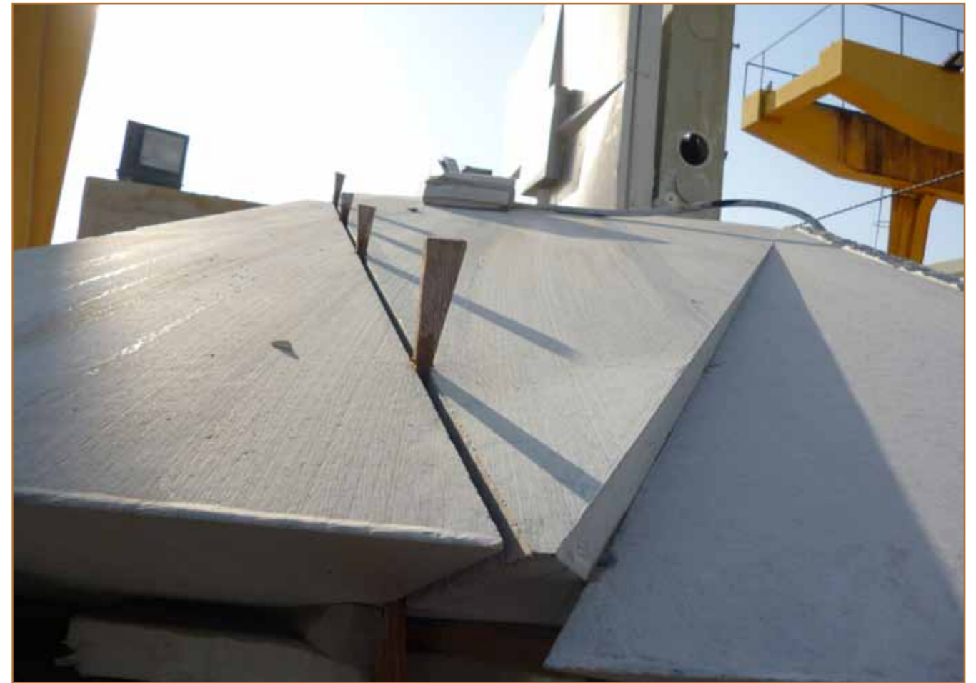
Detailed view to splitting process (Workshop in Aswan)
