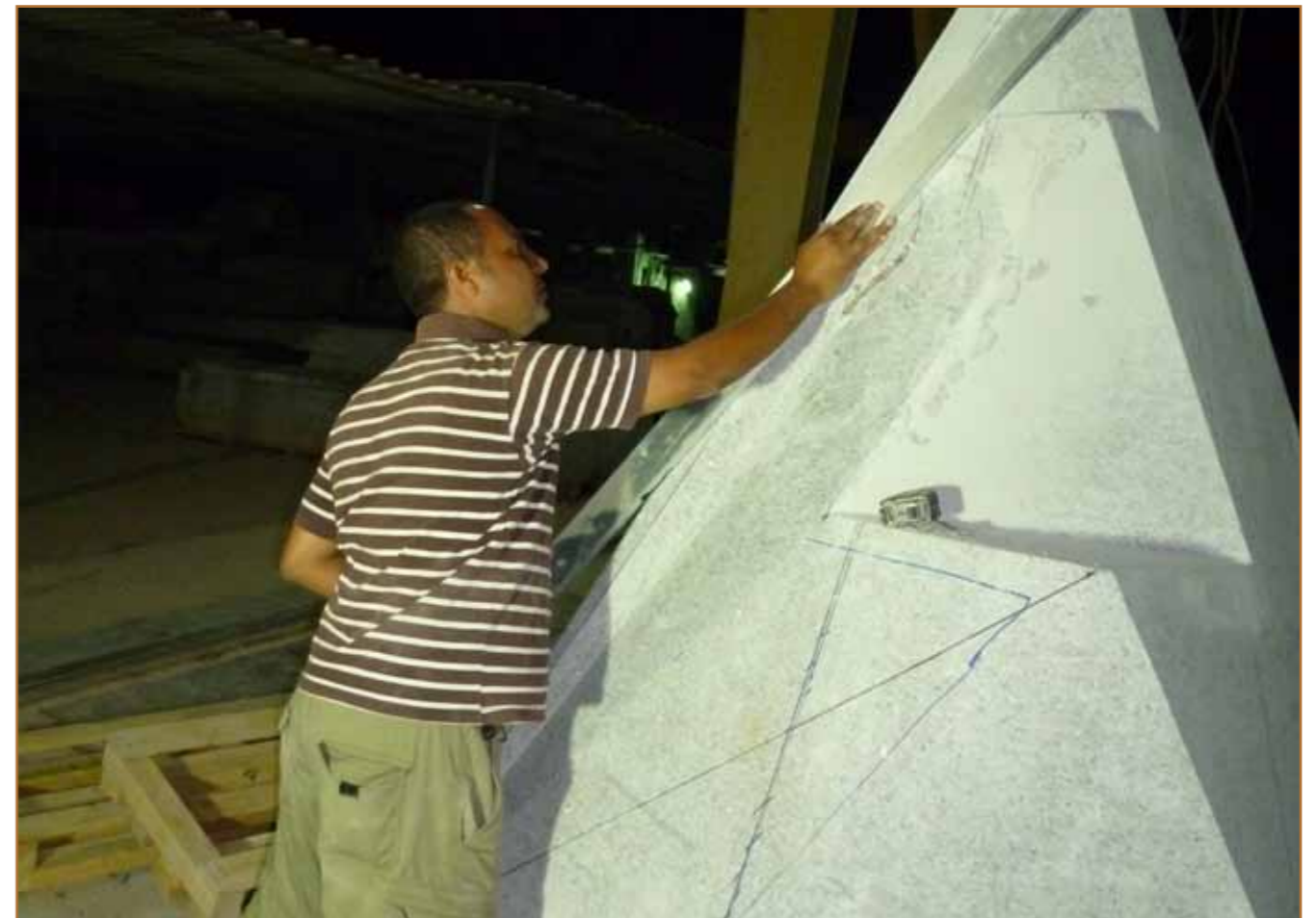
Measuring "diamond side" before cut progress (Workshop in Aswan)
