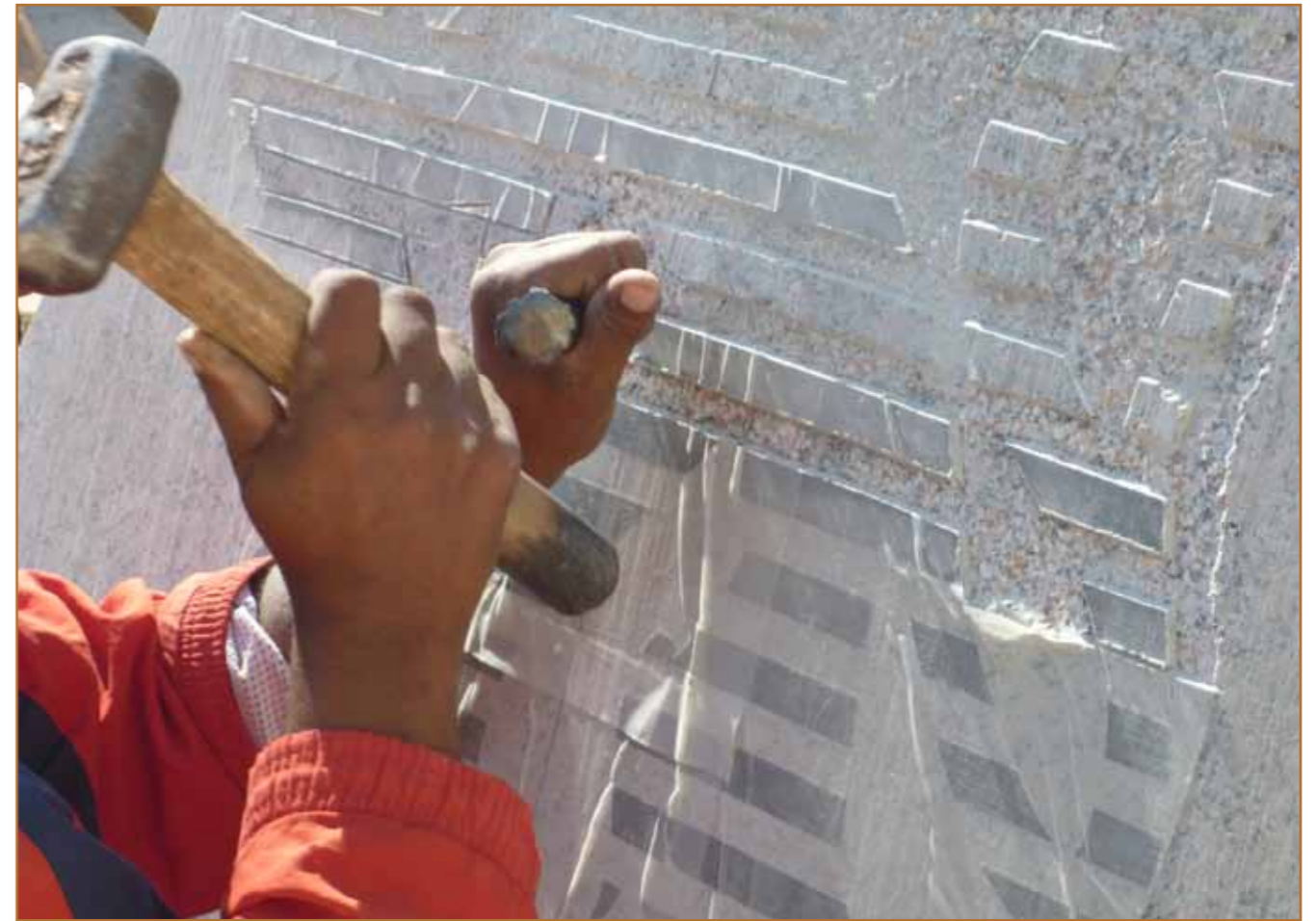
Hammering to achieve different level deepness of design (Workshop in Aswan)
