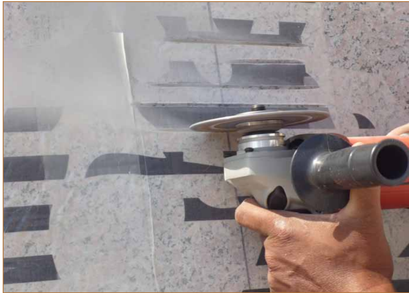
Cutting by power tool first shape of design to granit stone (Workshop in Aswan)
