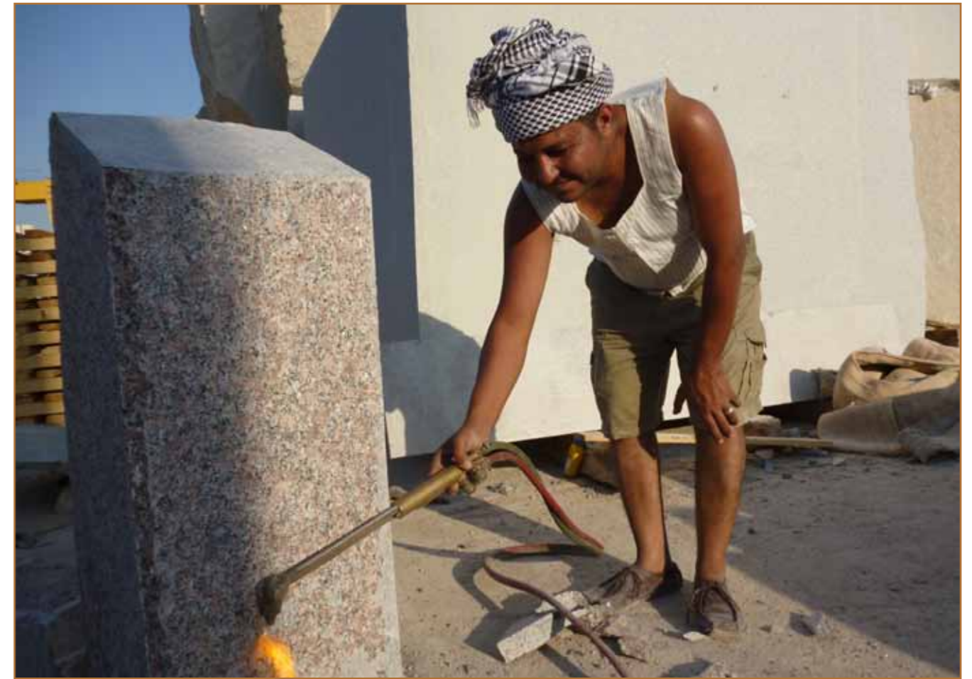
High temperature flame applied to desk stander (Workshop in Aswan)
